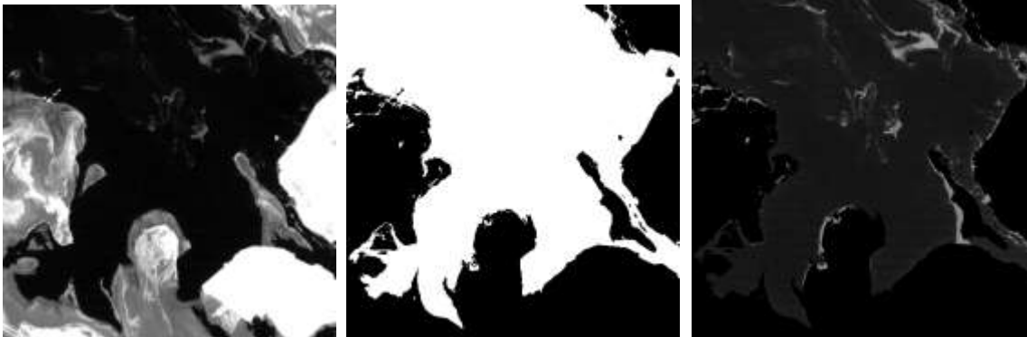
Figure 3. Black and White, unmodified image of TM Band 5 (left), TM band 4 land/water mask (mid), and the resulting multiplication of TM band 5 to the TM band 4 land/water mask (right). Oil slicks with high spectral reflectance stand out among the low-reflectance water features and the masked-out land features.
